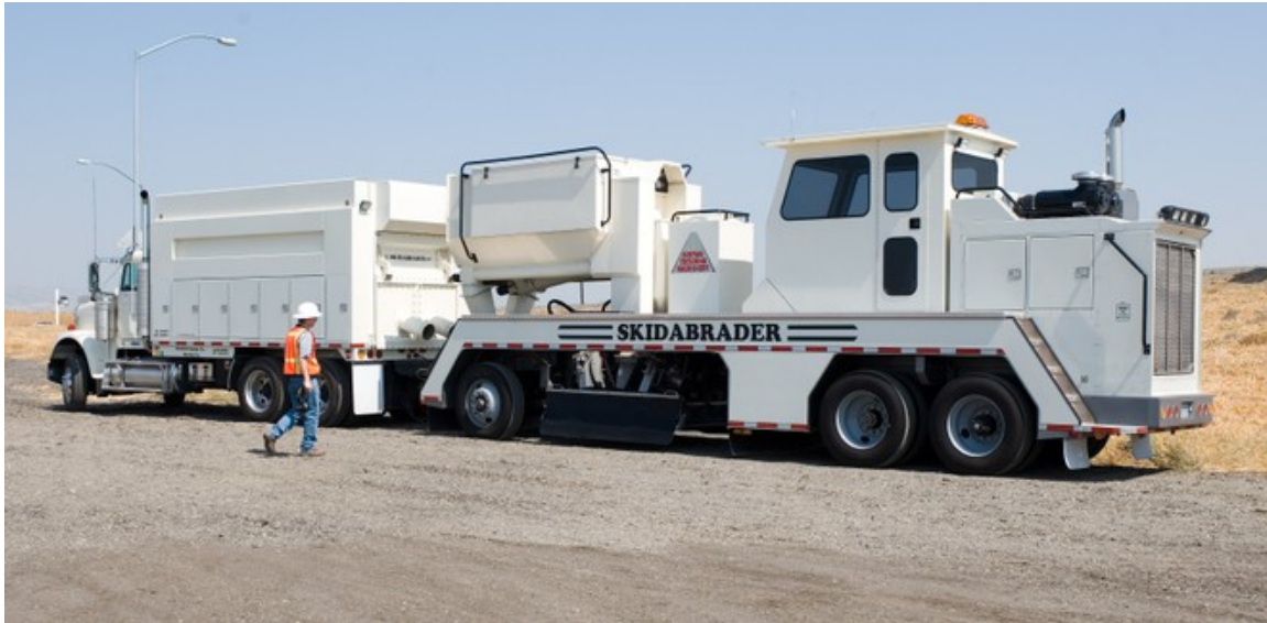
Figure 1. Skidabradar® equipment used to shot peen pavement. The rear vehicle shot peens the pavement and pushes the forward vehicle which vacuums the road dust and shot and extracts the shot for recycling.
