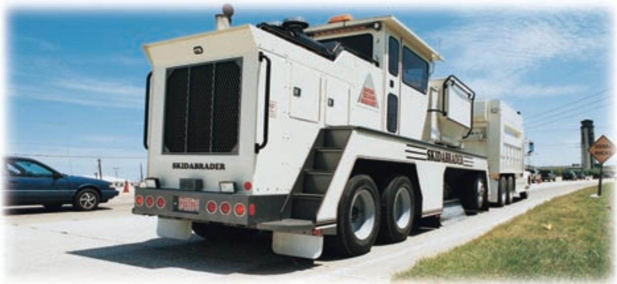
**T**he SKIDABRADER is designed to texture pavement surfaces. It recycles steel abrasive media utilizing the high velocity impact method to produce a six-foot wide swath of textured surface in a single pass. It is the most productive machine of its type, providing the fastest, simplest, and cleanest way to modify pavement surfaces. The texture depth can be infinitely controlled on asphalt, concrete, and other surfaces. It is a completely dry and dust-free process that requires no cleanup.
