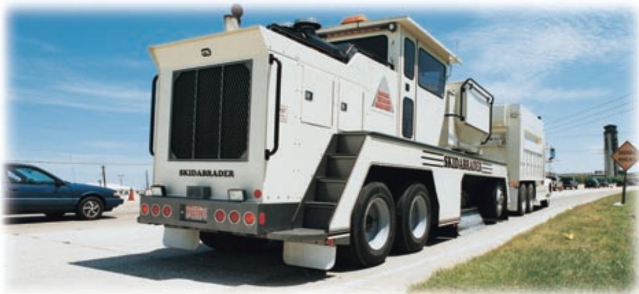
**T**he SKIDABRADER is designed to texture pavement surfaces. It recycles steel abrasive media utilizing the high velocity impact method to produce a six-foot wide swath of textured surface in a single pass. It is the most productive machine of its type, providing the fastest, simplest, and cleanest way to modify pavement surfaces. The texture depth can be infinitely controlled on asphalt, concrete, and other surfaces. It is a completely dry and dust-free process that requires no cleanup.
