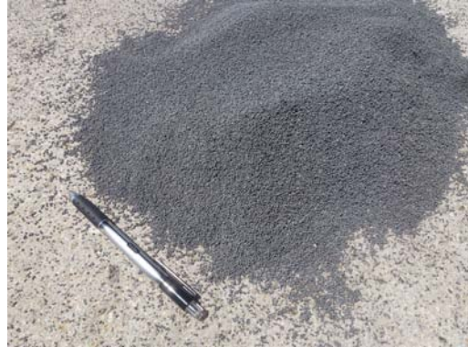
No. 390 steel shot blast used in the Roswell Skidabrader treatment.
