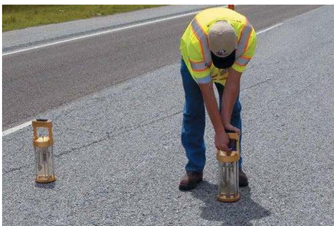
Directly behind the surface texturing procedure macro texture evaluation at three tests per lane mile were performed using the specified outflow meters
